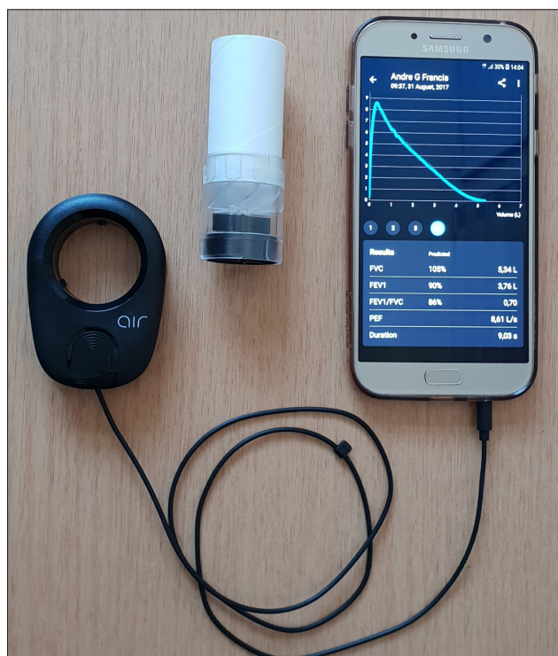
Fig. 1. The Air-Smart Spirometer (Pond Health Care Innovations, Sweden), connected to a standard smartphone.
